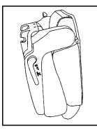
Lift the lever again to release the rear of the seat from the floor. The seat will tumble forward. Folding and Tumbling the Seat(s) from the Third Row Seats
